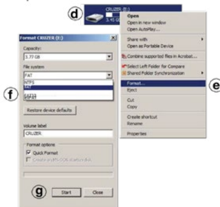
Figure 10. Formatting Memory Device to FAT
