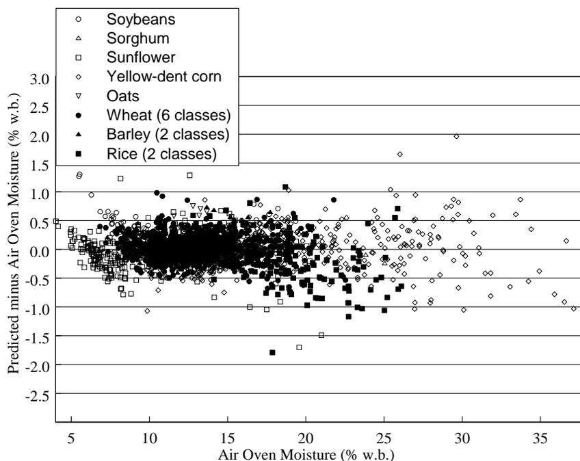
**Figure 2. Predicted moisture measurement error for 15 grain types and 3 crop years with the unified moisture algorithm. (Funk, 2001)**
