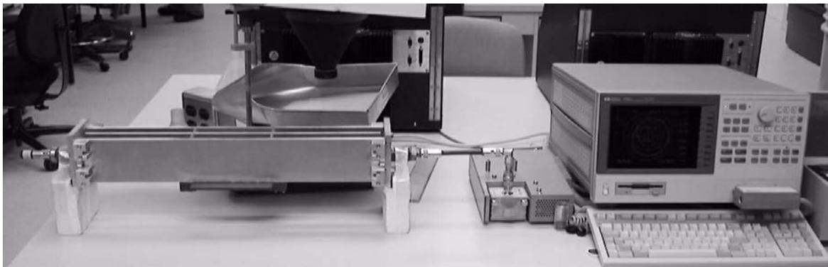
**Figure 1. Transmission line test cell and HP-4291A RF Material/Impedance Analyzer**
