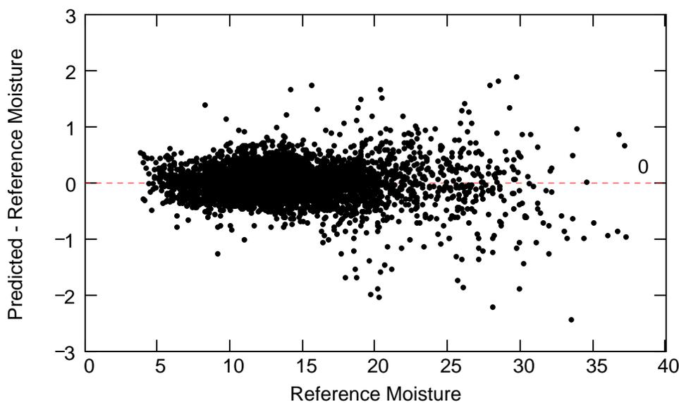
**Figure 5. Performance of the Unified Moisture Algorithm (predicted minus reference moisture) for 5,141 samples representing 53 types of U.S. cereal grains, oilseeds, pulses, and processed rices for the 1998-2002 crop years.**
