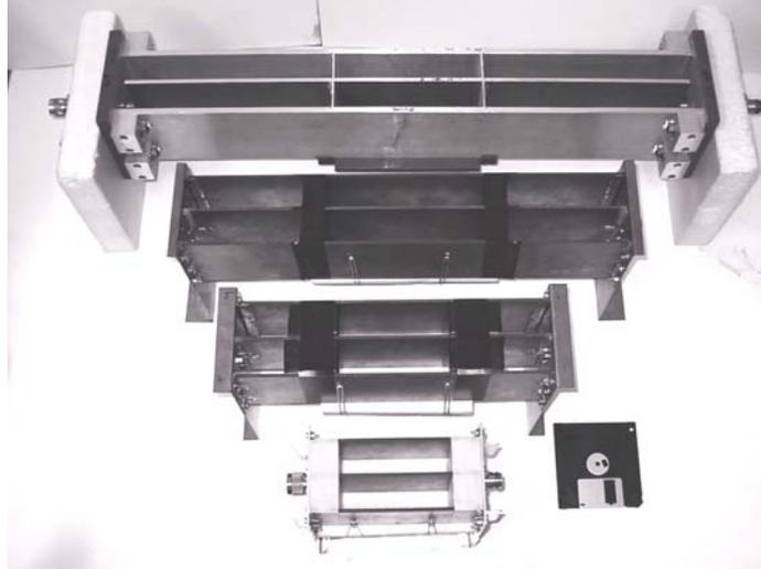
**Figure 4. Four prototype test cells that were created to test the feasibility of obtaining compatible results with different sizes of test cells. (with diskette for size comparison)**
